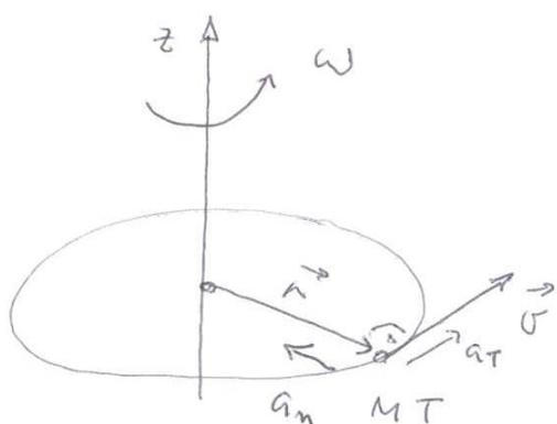
$$v = \omega r \quad (\vec{v} = \vec{\omega} \times \vec{r})$$
