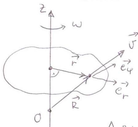
$$\begin{aligned} d\vec{L} &= dm \vec{R} \times \vec{v} = dm (\vec{ze}_z + \vec{re}_r) \times \omega \vec{re}_\phi = \\ &= -dm \cdot z \vec{re}_r + dm r^2 \omega \vec{e}_z = \\ \vec{L} &= -\vec{we}_r \int dm \cdot z r + \vec{we}_z \int dm r^2 \end{aligned}$$
